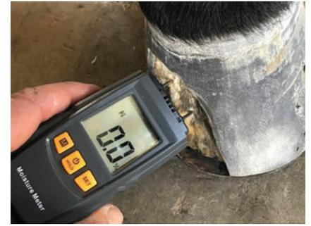
2. The prepared area is dried with a heat gun to maximize the bond. Drying is monitored with a FootPro™ Moisture Meter to get the surface moisture level below 10%. Ideally, zero percent moisture is desirable, and was achieved this time.
